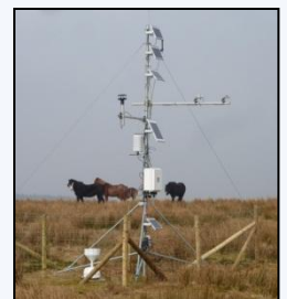
Automatic Weather Station data from Llyn Brianne at 15 minute resolution is available to view online .
